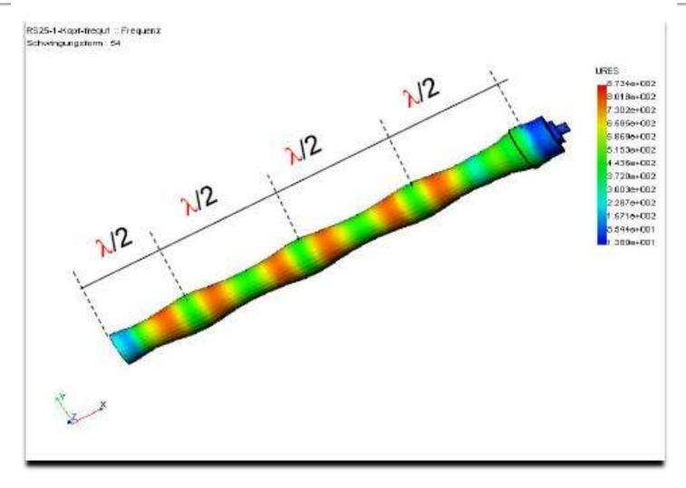
Power rating for resonation depends on the length of the resonator
